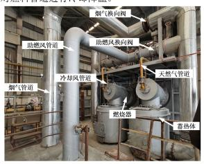
图 1 蓄热式熔铝炉燃烧器侧实体结构 Fig. 1 Structure of burner side of regenerative aluminum melting furnace
