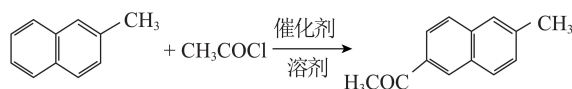
图4 2-甲基萘和乙酰氯酰化合成2-甲基-6-乙酰基萘 Fig.4 Synthesis of 2-methyl-6-acetylnaphthalene by 2-methylnaphthalene and acetylchloroylation
