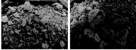
a) w(\text{神华煤}) : w(\text{石炭煤}) = 1 : 1 b) w(\text{神华煤}) : w(\text{石炭煤}) = 3 : 1
